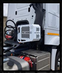
THE DELTA OIL COOLER IS A COMPACT, SELF CONTAINED, HYDRAULIC DRIVE UNIT DESIGNED FOR USE ON COMMERCIAL VEHICLES. IT IS LIGHT-WEIGHT, MAINTENANCE FRIENDLY AND UTILIZES A MINIMAL AMOUNT OF HYDRAULIC OIL. KEEPING ENVIRONMENTAL AND SERVICE COSTS TO A MINIMUM.
